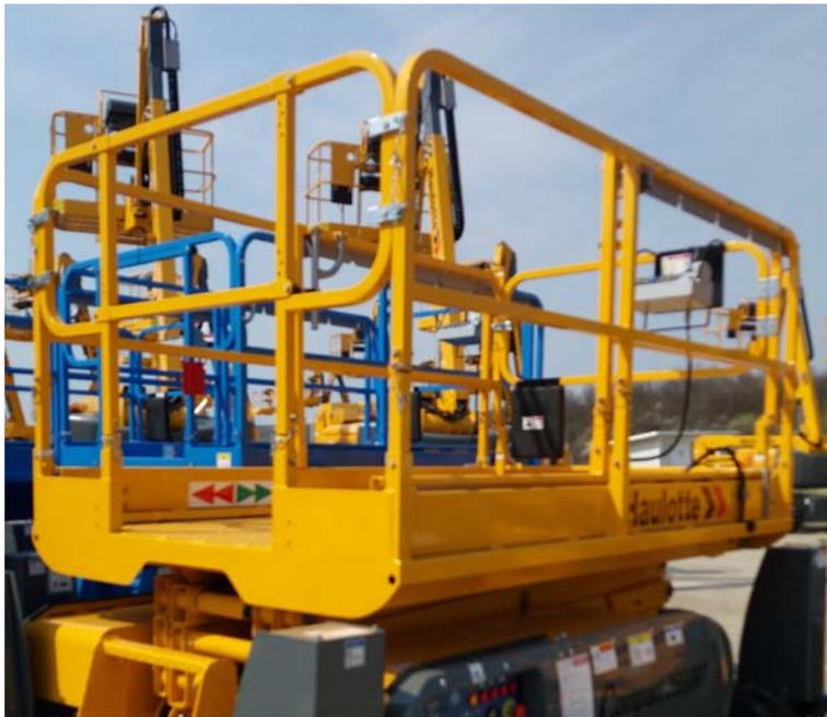
Remove platform control box from its designated position and place it on platform floor
