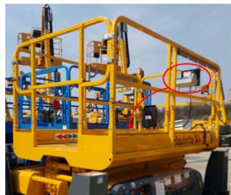
Remove the 2 pins (G2) from the platform front guardrails.
