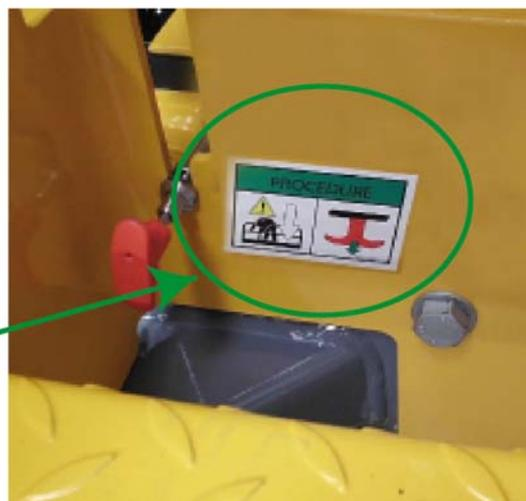
***N.B.:-PULLING ON TO THE T-HANDLE, IMMEDIATELY ACTIVATES THE EMERGENCY LOWERING OF THE PLATFORM.***
