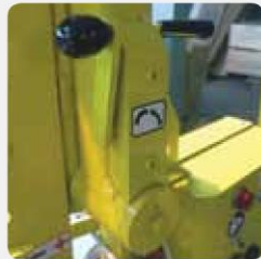
Tilt & rotate handles
