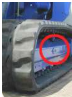
Fig. 66 The nut for the tension roller is placed here
