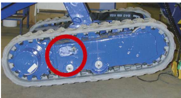
Fig. 66a The nipples for the tension roller is placed here
