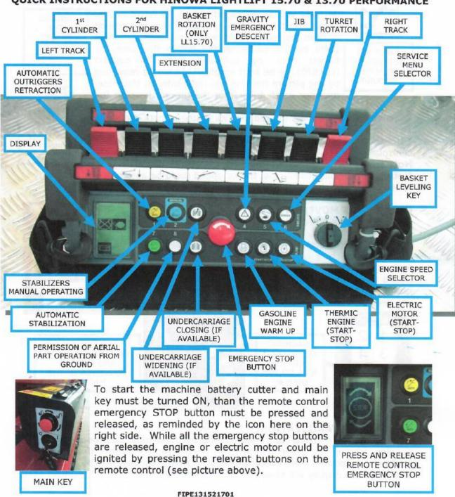
**Note1:** On gasoline machine when the engine is cold, once it's ignited, it's possible to warm it up pressing the "WARM UP" button on the remote control, engine will run faster for 20 seconds.
