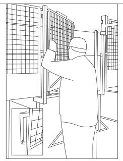
The Access Gate should now be placed in the proposed access bay ensuring the gate opens to the right and inwards towards the working platform. Fasten the locking thumb screw on to the lower elongated hinge pin to prevent accidental removal of the access gate (Inset). (NB: A Bridging Deck MUST aways be used on the same bay as an Access Gate.)
