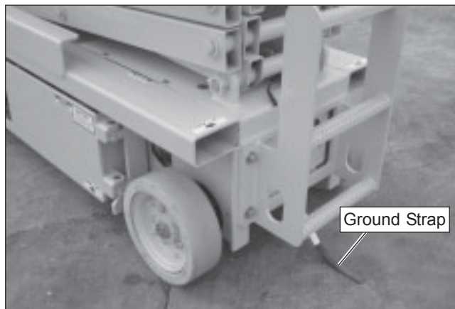
Figure 8.10 – Rear of Chassis
