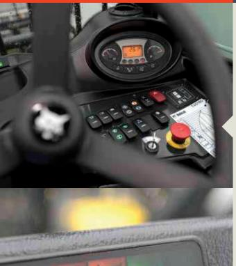
FNR on Joystick puts maximum control at your fingertips. Select the driving direction at the touch of a button, while still keeping a grip on both the steering wheel and the joystick for improved safety and productivity.
