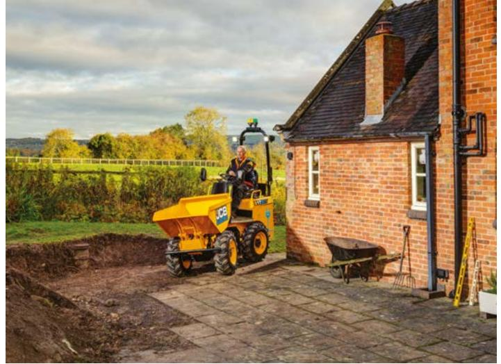
With 7kW continuous and 20kW peak power, the ITE matches the performance of its diesel counterpart.
