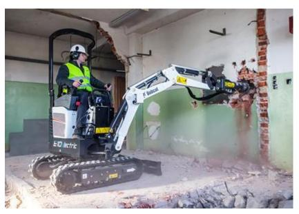
Bobcat has launched the world's first 1 tonne electric mini-excavator at Bauma 2019. Combining zero emissions, low noise and a width of just 71 cm, Bobcat's new E10e battery-powered, zero tail swing (ZTS) mini-excavator can easily pass through standard doors and in and out of lifts, making it ideal for indoor applications such as demolition and basement construction.
