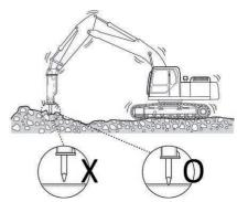
Conversely, if thrust is excessive or breaking is performed with boom of the carrier raised as shown below, the machine may suddenly tip toward the movement. The breaker body may strike the broken rocks violently resulting in damage.
