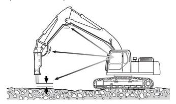
**Stop as soon as breaking is completed.** As soon as rocks are broken, cease power to the breaker. If idle striking continues the accumulator may be damaged, the bolts loosened or broken and also damage may be caused to the excavator. When a proper thrust is not applied to the breaker or the tool is used as a lever, the state of idle striking will occur. (Idle striking makes a higher pitched ringing sound).
