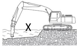
**Never use the breaker as a sledge hammer.** Before starting up, rest the breaker on the ground. Never attempt to use the breaker and excavator boom as a sledge hammer to break material. This will damage parts of the carrier.
