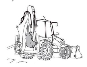
Backhoe Loader with breaker in travelling position
