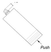
2. Insert the cartridge and turn clockwise to hand tightness only.
