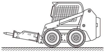
Skid Steer Loader with breaker in travelling position
