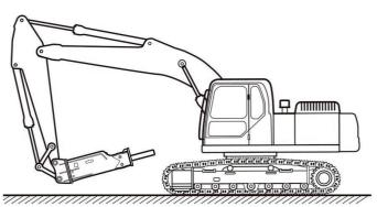
Excavator/Compact excavator with breaker in travelling position
