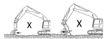
**Never lever with the breaker**. Never attempt to use the hydraulic breaker as a crowbar. The breaker is not designed for lateral loads. Both breaker and tool will be damaged.
